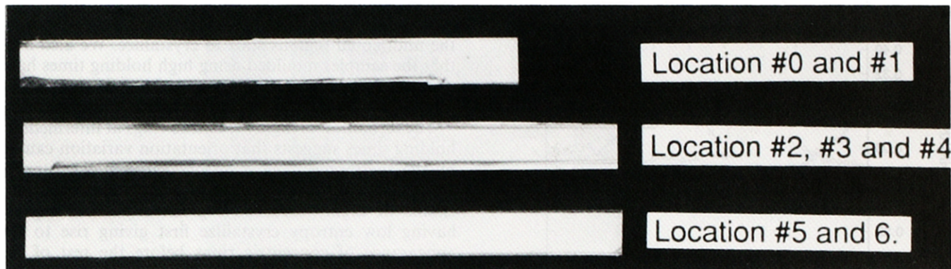
Figure 5 Transmission optical photomicrographs of a B-cut sample moulded at 20°C using the low injection moulding speed
